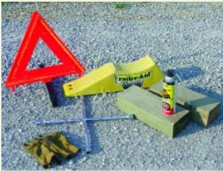
**Tire changing tools: leather tools, star lug wrench, trailer tire changing aid, wood tire block, emergency tire sealant, emergency road triangle, and flashlight. Don't forget the spare tire, as well.**
