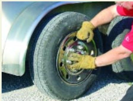
Replace the wheel cover, ensuring that the valve stem opening is properly lined up. Line up the cover so that it almost pops on the wheel. Then, using your gloved fist, firmly tap the portion that is not snapped. It will pop into place. Tap around the cover to ensure that it is firmly in place.
