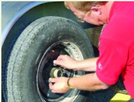
Insure that the tire is pushed all the way back onto the hub. put the lug nuts back on the lugs and tighten to finger tight. Next, tighten the lug nuts with the star lug wrench in an alternating pattern. Start with the top nut, next do the bottom nut, then the nut at the upper left, then lower right, etc. This cross-type pattern will help ensure the wheel is lined up correctly on the hub.
