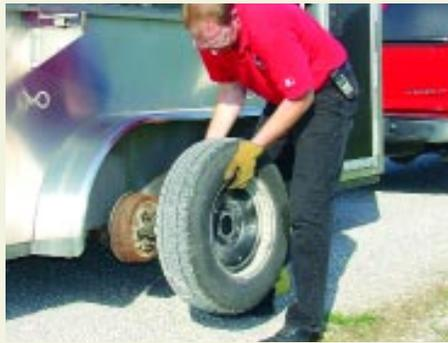
Lift the flat tire and wheel off the hub and set it aside.
