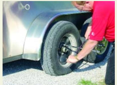
**While all trailer tires are still on the ground, use a star lug wrench and loosen all the lug nuts on the flat tire wheel. (Note: if you raise the tire off the ground before loosening the lug nuts with the wrench, they are very difficult to break loose because the wheel will spin freely.) Leave them finger-tight still holding the wheel on the trailer.**
