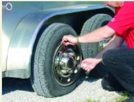
**Using a large flat screwdriver, remove the wheel cover from the flat trailer tire.**
