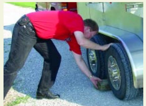
**Set the wood wheel blocks in front and back of the tires on the opposite side of the trailer to help prevent rolling.**
