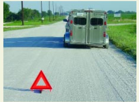
**Whenever possible, pull off the highway onto a side road, choose a location with lots of site distance, and set the emergency flashers and set out the emergency triangle.**
