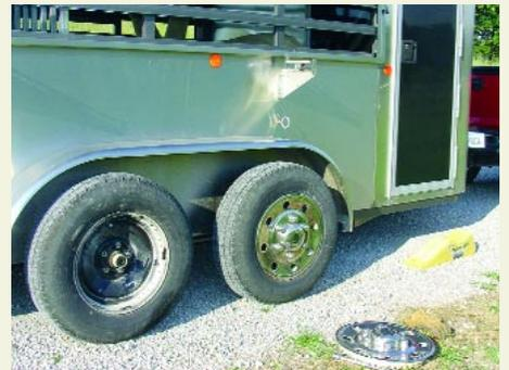
Remove the wood tire blocks. Back down off the trailer tire changing aid.
