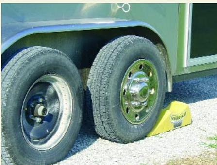
**Place the trailer tire changing aid in front of the good front tire on the same side of the trailer as the flat tire. This way, you can pull onto the aid. If the front tire of the trailer is flat, place the trailer changing aid in back of the good back tire and back onto the aid.**
