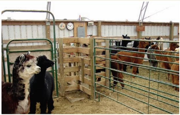
Hoop buildings offer great flexibility because they have a totally clear floor area, free from building columns. An automatic waterer, strategically located in the center of the building, is accessible by animals in up to four pens. A clay floor allows the Post family to reconfigure the pen layout throughout the year.
