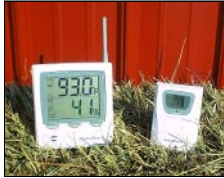
Wireless temperature and humidity monitoring equipment is simple to install and invaluable for transporting in hot weather. The temperature and humidity sensor is easily mounted in the trailer (no wires to run), and is very accurate.
