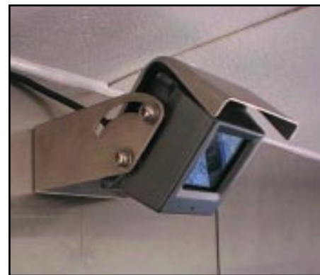
The three inch camera covers a wide, 130-degree angle, has a stainless steel mounting bracket, is water-resistant, and handles road vibration very well.
