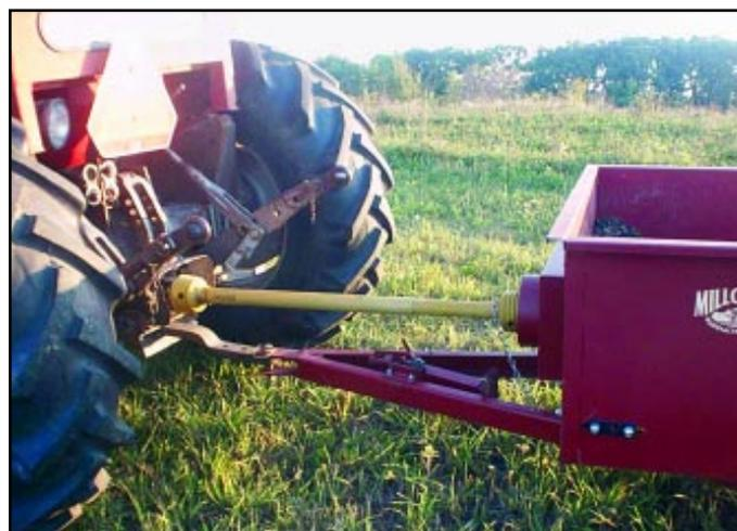
Medium-sized spreaders can be pulled by utility tractors and are designed to be ground driven or powered by a power take-off (PTO) shaft. The PTO shaft is used to transfer the power from the tractor engine to the spreader to drive the manure spreader system.
