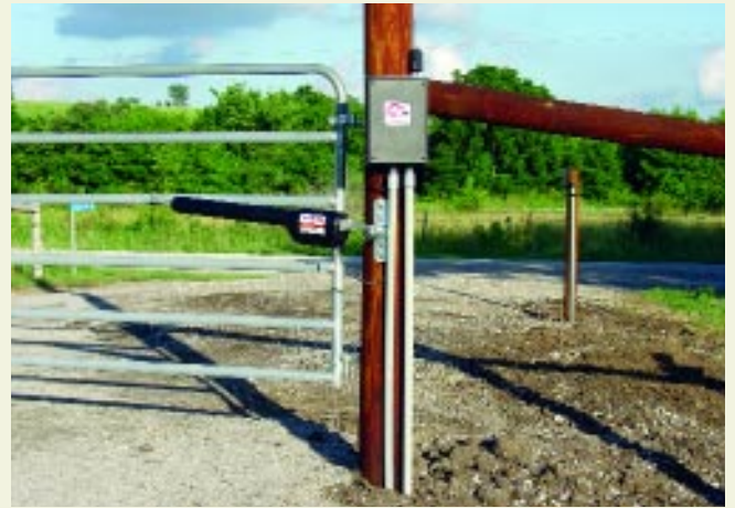
2. An automatic gate opener is a mechanical device that swings a driveway gate open when activated by an electric impulse from a remote control device, and electronic keypad or a sensor mounted in the edge of the driveway.
