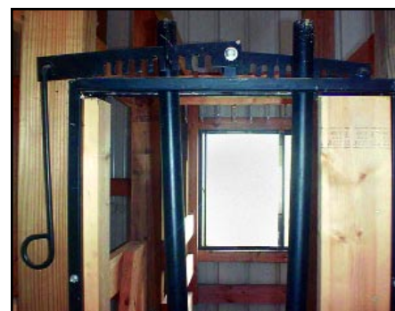
A head gate should be designed to be adjusted easily and quickly. Alpaca necks vary greatly in thickness. Even the same alpaca's neck varies from full-fleeced to shorn condition. This head gate can be adjusted easily by one person.
