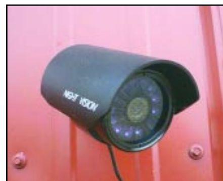
Cameras come in a wide variety of types and price ranges. This one is black and white, weatherproof, with a wide angle lens, infrared, and night vision capability. It works great in a barn, under a shed roof, or in an outside pen.
