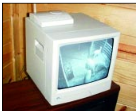
This CCTV monitor is a stand-alone unit with a high quality picture. On the top is a receiver/switcher used to receive wireless transmissions and rotate the pictures from several cameras.
